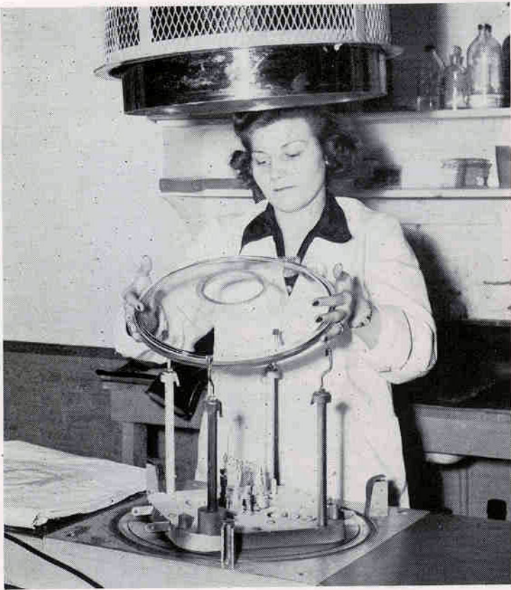
9. The spherical mirror which forms the main "lens" in the reflective optical system is shown here before aluminizing. It is a salad-bowl shaped piece of glass 14 inches in diameter with a 4-inch hole in the center. The inner surface is ground to a true spherical shape on a standard optical grinding machine.
