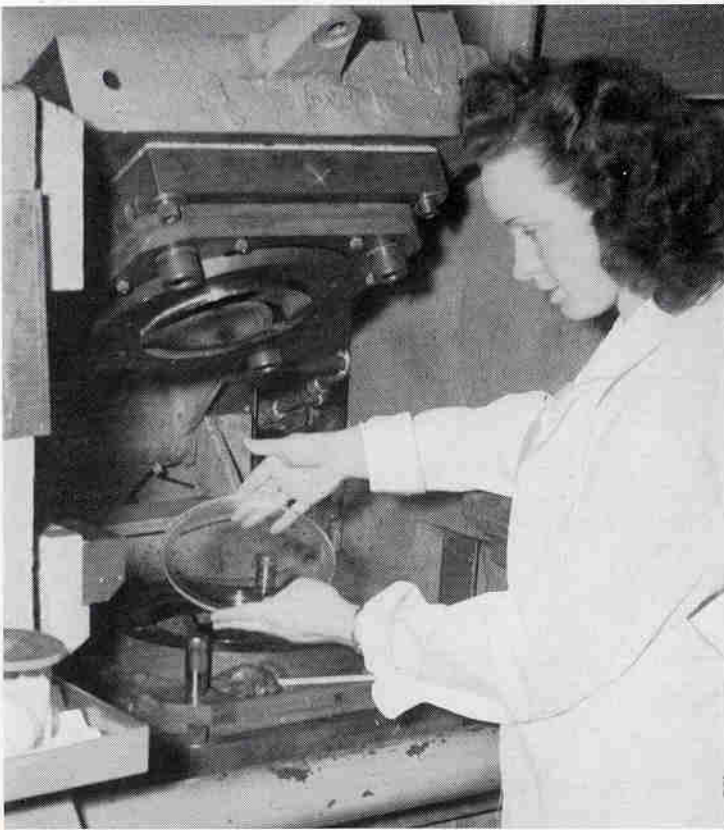
7. When the mold has cooled to near room temperature, the press is opened and the fully shaped lens removed. Except for boring the hole in the center for accommodating the neck of the projection tube, the lens is ready for use as it comes from the mold. No polishing or finishing of any kind is required.
