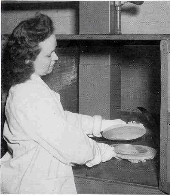
5. A methyl-methacrylate disk, 8 inches in diameter and \frac{1}{4} inch thick, is placed between metal electrodes connected to a radio-frequency power generator. Application of power (1 KW) for 3\frac{1}{2} minutes heats the disk to a temperature of 150^\circ throughout. The electrodes are located in an interlocked, screened enclosure
