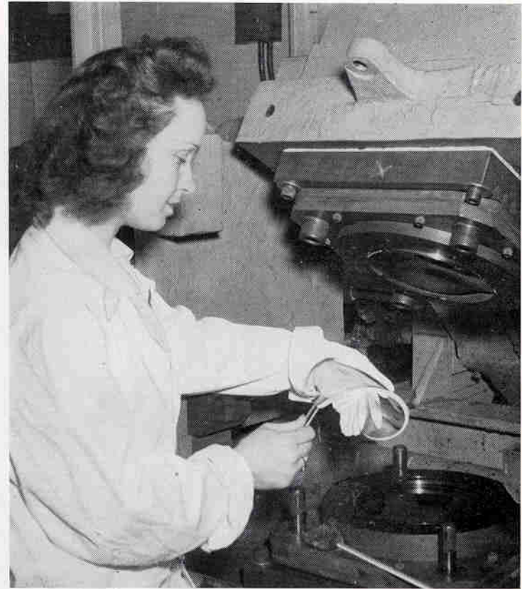
6. The heated disk (usually referred to as a "preform") is soft and flexible as it comes from the radio-frequency preheating cabinet. The molds, heated by steam pipes, keep it soft during pressing. When the heating cycle is completed, steam is shut off and cold water turned on.
