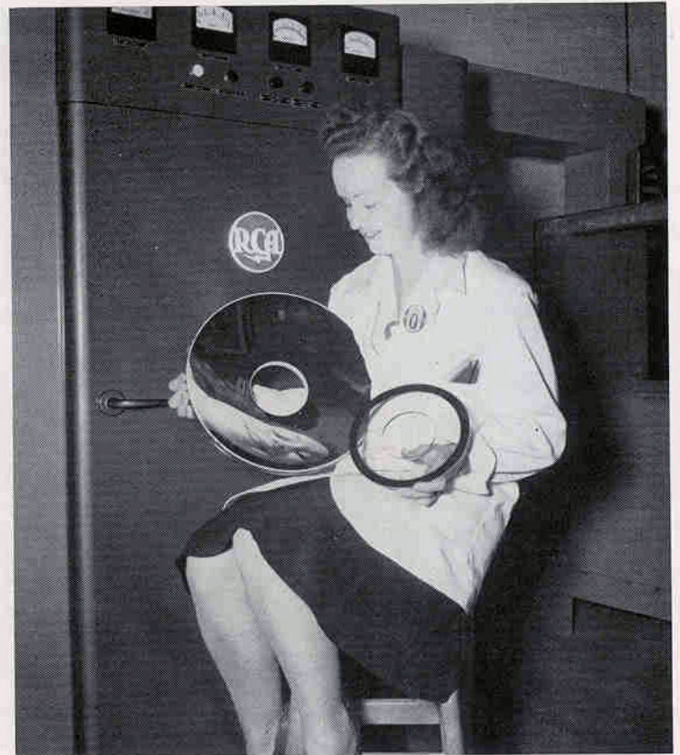
12. The two lenses, completed and ready for mounting in the projection-type home receiver. In the background is the standard RCA Type 15-B Radio Frequency Generator used in preheating the plastic disks before molding. At the right rear is the screened enclosure containing the heating electrodes.
